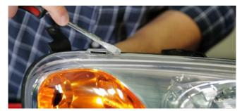
Heat up the next 6-8 inches along the seam, and again use the screwdriver to break the seal. Pry outward on the lens VERY gently from time to time as you feel the lens become looser. Remember you are working with plastic, and it is possible to melt, burn, and crack it if you don't exercise care and patience. Continue to work in small increments of 6-8 inches at a time. You can use a second screwdriver to wedge between the housing and the lens during this process, however it is not
